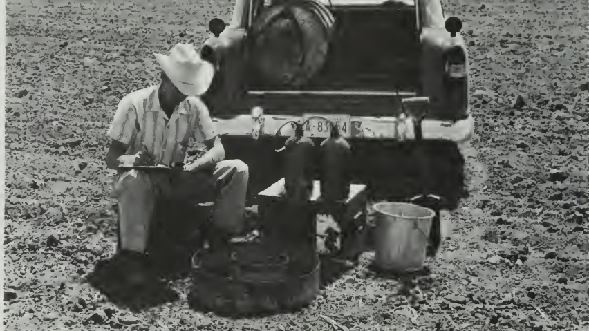
A device for determining how fast water enters the soil. This knowledge is necessary for planning irrigation or terraces.
